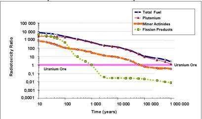
Diagram 2 : Simplified chart of the evolution of the radiotoxicity of spent nuclear fuel and of its components
