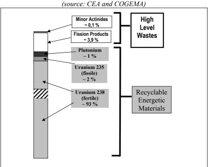
Diagram 1 : Composition of unloaded irradiated fuels of the UOX type (uranium oxides) as a % of their total mass (source: CEA and COGEMA)
