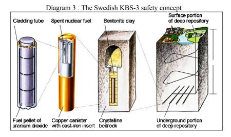
Lastly, the copper canisters are surrounded, when stored, by bentonite clay ( $5^{th}$  barrier) impervious to water and which immobilises radioelements.
