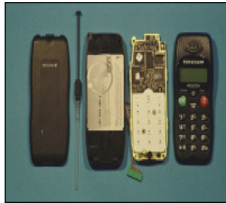
Exploded of a mobile phone - Source : CNRS
